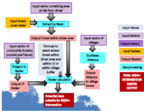
Workflow for Intervention SIMPLISTIC HYPOTHETICAL EXAMPLE FOR TECHNICAL DEMONSTRATION OF ARCGIS MODEL BUILDER ONLY
