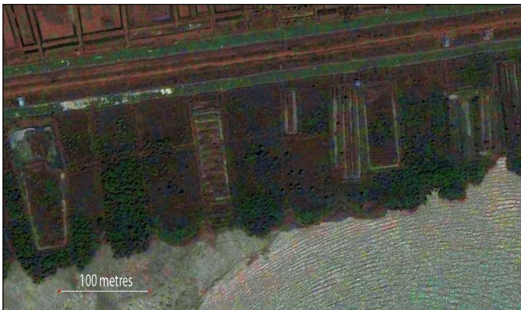
Figure 80: Degraded mangrove with unused aquaculture ponds, Kien Luong. Note a lack of tree cover and the eroding front of the mangrove. Erosion appears apparent even where mud extends out to sea (left of picture) (Image: Google Earth). The thickets in the non-treed areas may be suppressing regeneration.
